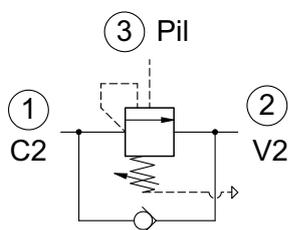
The Vented counterbalance valve has a vented spring chamber. Both the relief and the pilot opening of the valve are independent from backpressure at port 2. These valves must be used only in conjunction with directional valves with closed center spools and equipped with port relief valves. This version of counterbalance valve will be more efficient in systems with high backpressure or line losses between the counterbalance valve and the directional control.
