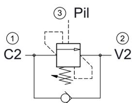
Port (1) is the load port; Port (2) is the exhaust port and Port (3) is the pilot port. The spring chamber on the NORMALE counterbalance valve is drained/connected to port (2). In this case, backpressure has effects on both the relief and pilot opening pressures since it pushes the relief piston in the closed direction and it opposes the pilot piston too.
